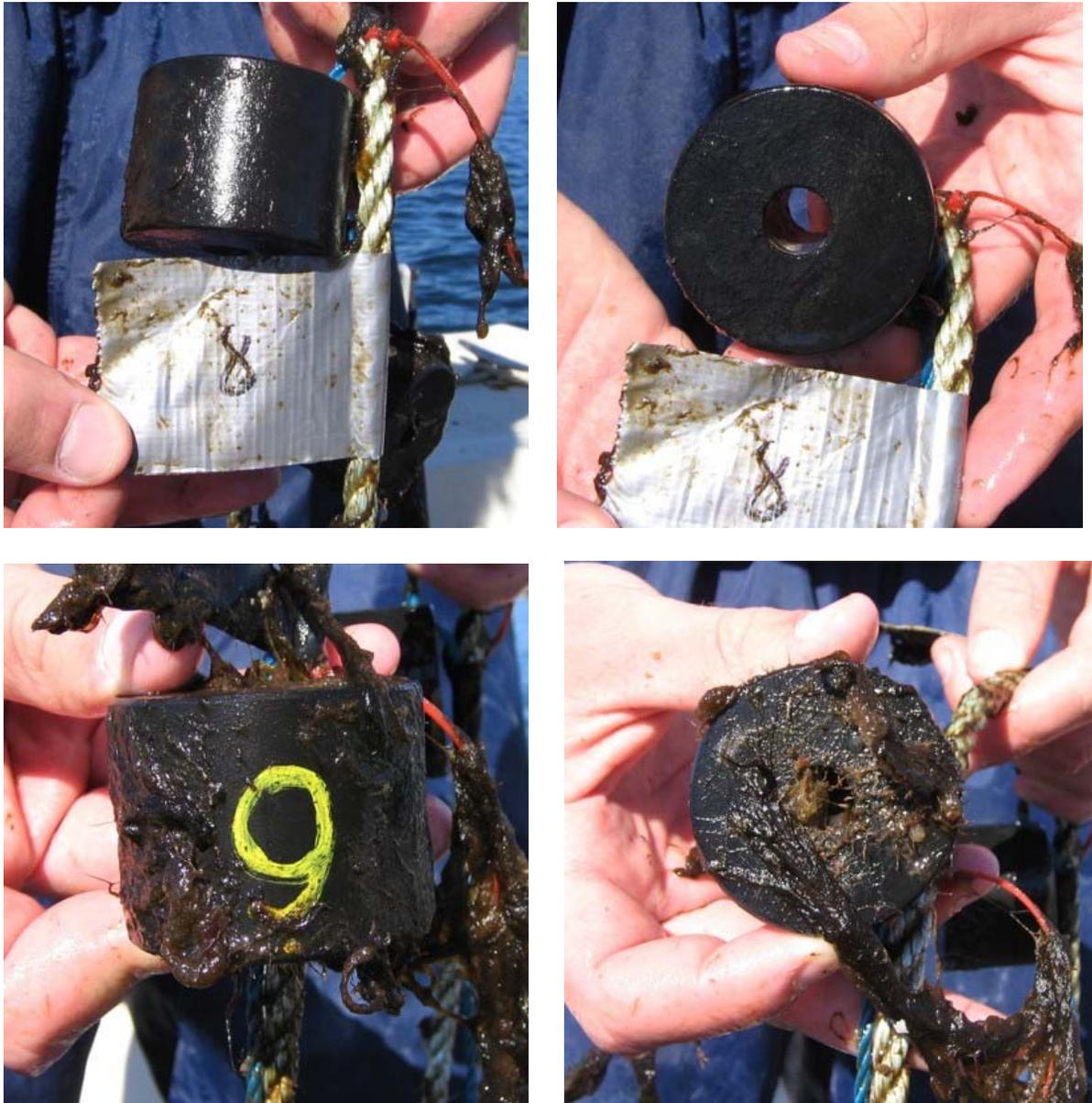
*Figure 3. Samples #8 (wax-coated) and #9 (non-coated) positioned close to each other at 10 inch after 3 month deployment period.*
