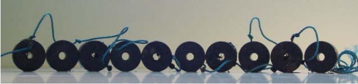
*Figure 4. The samples with the central holes view after receiving them back in RBR. From left to right: #1 – non-coated, #2 – coated, #3-non-coated, #4 –coated, #5-non-coated, #6-coated, #7-non-coated, #8-coated, #9-non-coated, #10 -coated*
